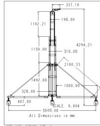
Fig. 9: Dimensional details of the mast
