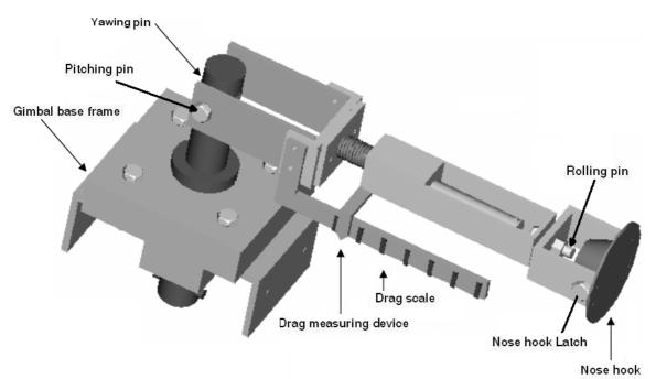
Fig. 3: Gimbal mechanism with different components
