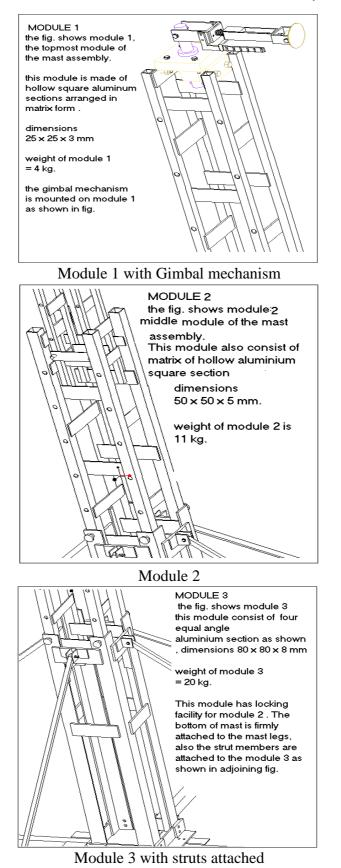
Fig. 4: The three component mast assembly
