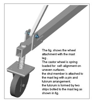
Fig.7: Spring mounted bolt for the castor wheel
