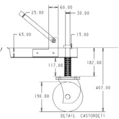
Fig.6: Details of castor wheel attachment
