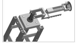
Fig. 8: Gimbal mechanism attached to module 1
