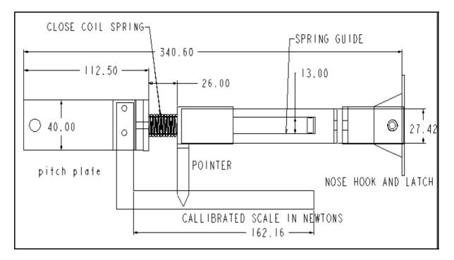
Fig. 3: Detailed drawing of the Drag Measuring and Alerting Device
