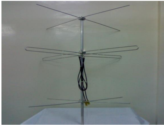
Fig. V: Yagi antenna at 145 MHz at IITB Ground station
