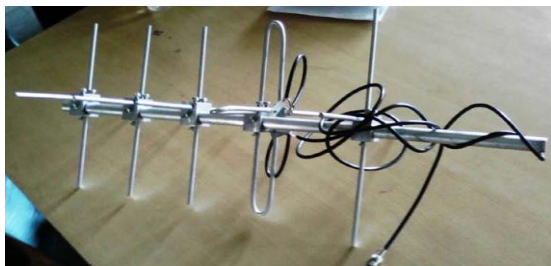
Fig. VII: Crossed yagi at 437MHz made by BVCOE Mumbai, India
