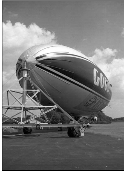
Fig 1: Mobile Tripod mast for Goodyear Blimp
