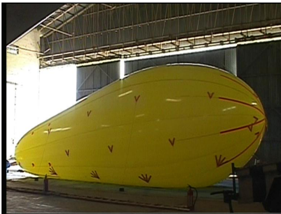
Figure 2. An inflated 100m 3 envelope of the aerostat
