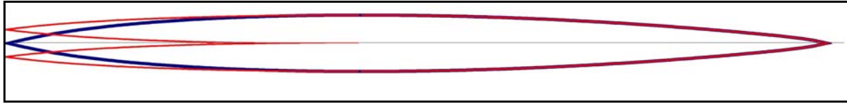
Figure 5. Conceptual sketch of single and split petal for envelope fabrication
