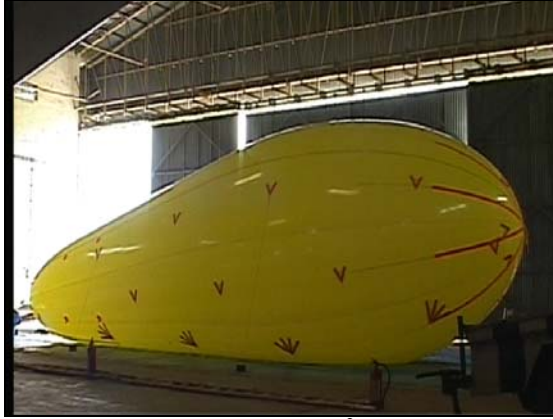
Figure 4. An inflated 100m 3 envelope of the aerostat
