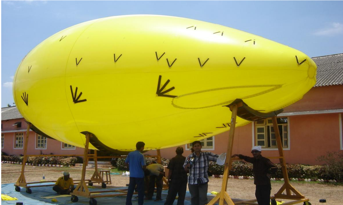
Fig 15: Aerostat being integrated and prepared for launch.
