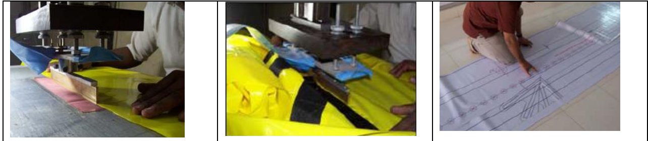
Figure 13: Snap shots of envelope fabrication process
