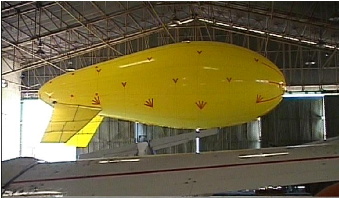
Fig 16: Aerostat filled with lighter than air gas ready for launch.
