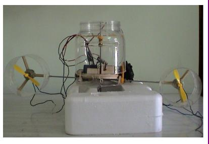
The motors were mounted in a pusher configuration for higher thrust. Balsa wood platform was made to support the receiver and servomotors. A four-channel receiver and transmitter kit (Futaba make) was obtained. Also a UHF Camera and Transmitter Set were attached to the gondola. Arrangement was made for easy replacement of the battery when the gondola is attached to the envelope.
