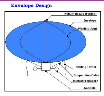
Survey of available literature suggested that the most appropriate shape for airships with good station keeping feature is the *Lenticular* shape, which is similar to a flying saucer, i.e., two dishes kept upside down on each other. But lenticular shapes result in large surface area, and lateral dimensions, hence the shape that was finally chosen is an oblate spheroid, i.e. an ellipsoid obtained by revolving the ellipse about its minor axis, as shown in the figure.
