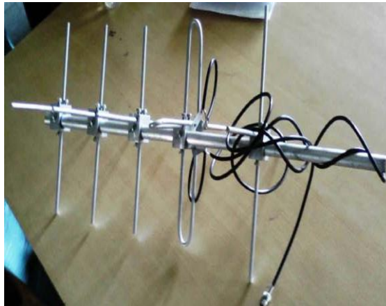
Figure 3: Crossed yagi at 437MHz made by BVCOE Mumbai, India
