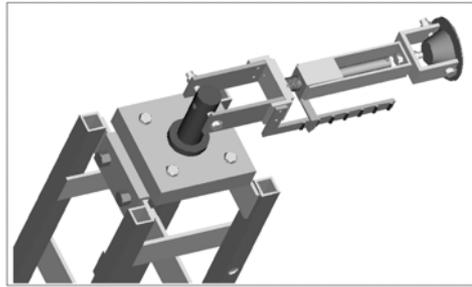
**Fig. 8: Gimbal mechanism attached to module 1**
