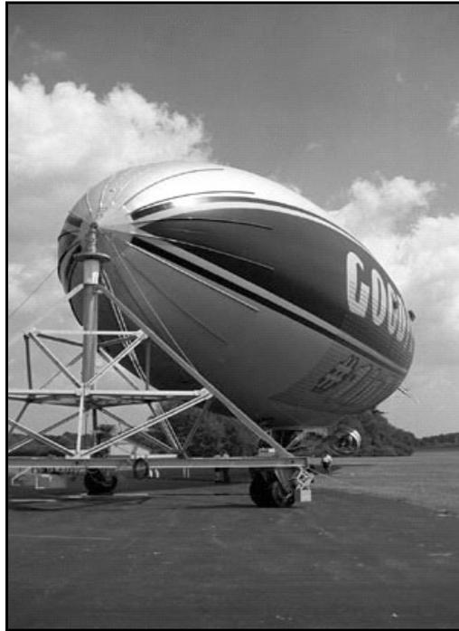
**Fig 1: Mobile Tripod mast for Goodyear Blimp**
