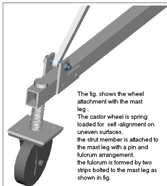
**Fig.7: Spring mounted bolt for the castor wheel**
