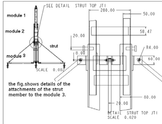
**Fig. 5: Dimensional details of strut attachment**
