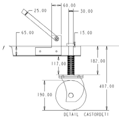
**Fig.6: Details of castor wheel attachment**
