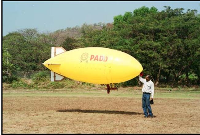
Figure 8 Micro Airship just before launch
