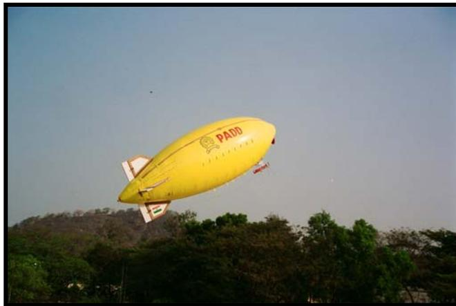
Figure 9 Micro Airship Just after Take off
