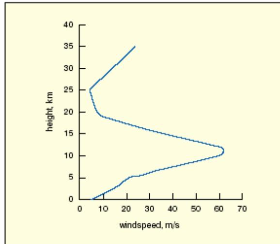
Figure 1. Typical Jet-Stream wind profile v/s altitude [1]
