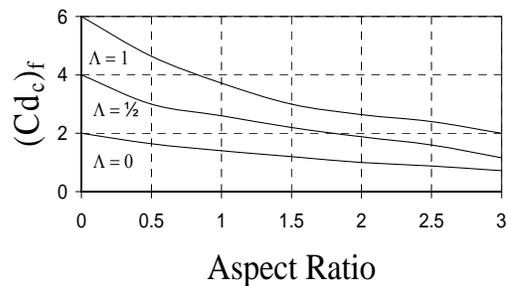
Figure 4 Fin Cross Flow Drag Coefficient
