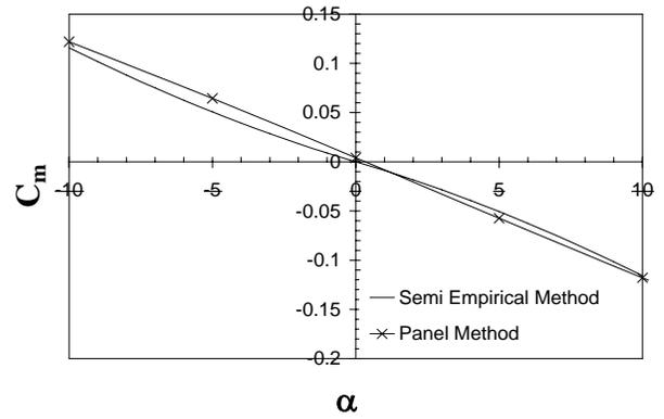
Figure 11 Moment Curve Comparison for GNVR Shape
