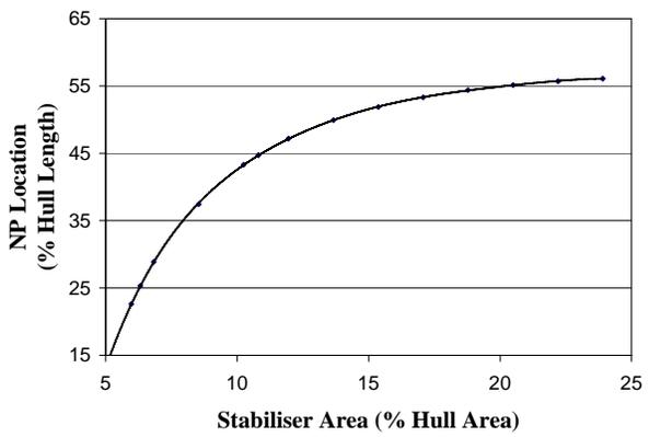
**Figure 14 Neutral Point Travel Due To Change in Fin Area (For SAC Shape)**
