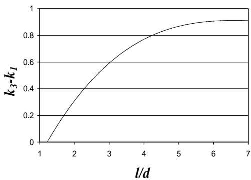
Figure 3 Lateral and Axial Apparent Mass Coefficient
