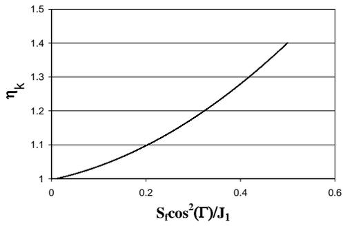
Figure 6 Hull Efficiency Factor
