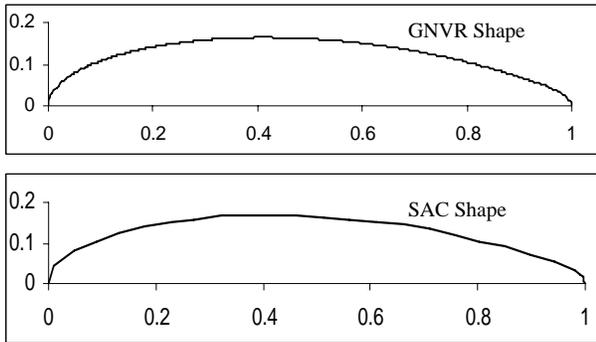
Figure 7 Hull Shapes for GNVR and SAC Configurations (only top half shown)
