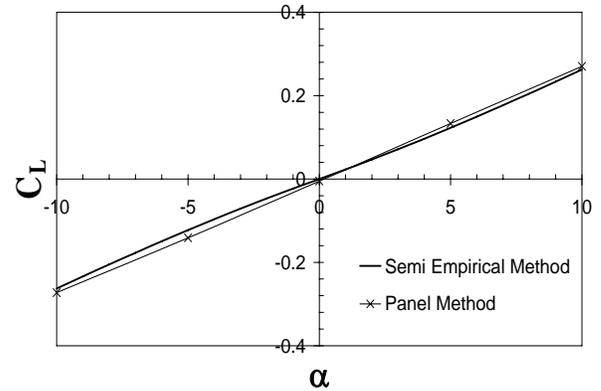
Figure 12 Lift Curve for GNVR Shape
