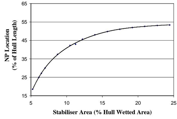
**Figure 15 Neutral Point Travel Due To Change in Fin Area (For GNV Shape)**
