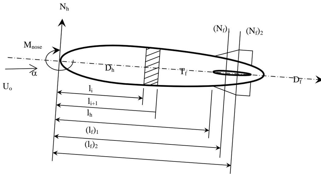
Fig. 1 Schematics of Airship Geometry, Forces and Moments
