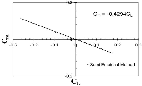
**Figure 13 Pitch Stability Coefficient Calculation from Semi Empirical method results for GNV Shape**
