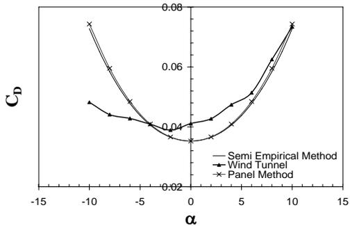
Figure 9 Drag Curve for SAC Shape
