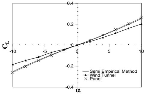
Figure 8 Lift Curve Comparison for SAC shape
