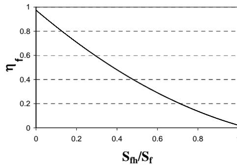
Figure 5 Fin Efficiency Factor
