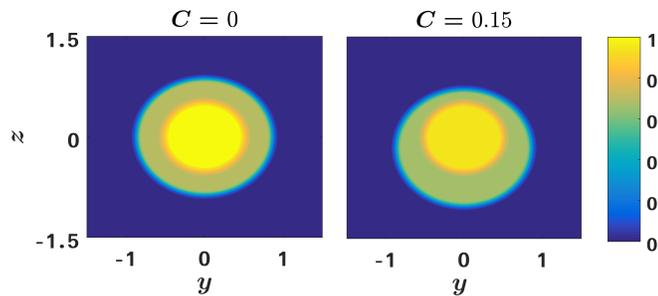
**Figure 1: Mean axial velocity  $u/U_p$  contours at  $x = 1$  station**
