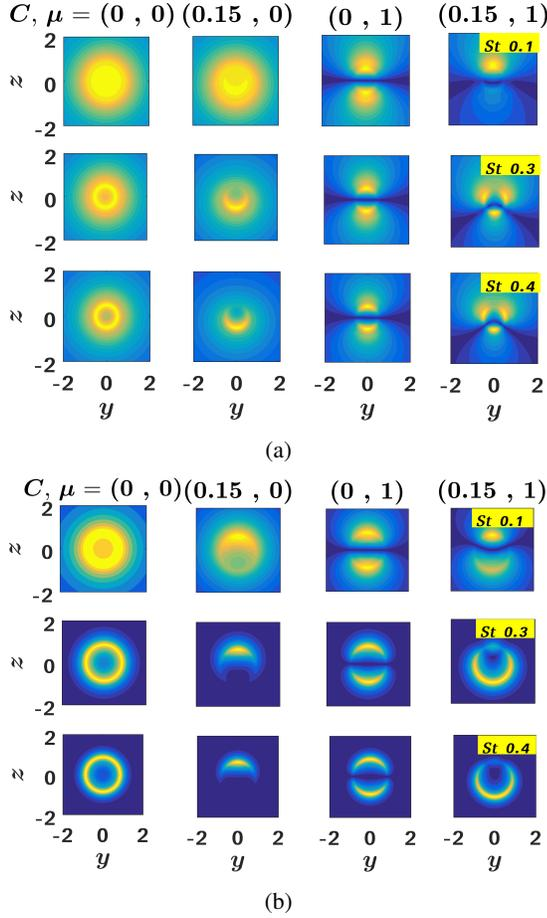
**Figure 4: (a) Inner mode pressure eigen function, (b) Outer mode pressure eigen function plots for concentric ( $C = 0$ ) and partially eccentric ( $C = 0.15$ ) jet at  $St$  of 0.1, 0.3 and 0.4 (arranged row wise). First two columns represents  $\mu = 0$  mode and last two columns represents  $\mu = 1$  mode.**
