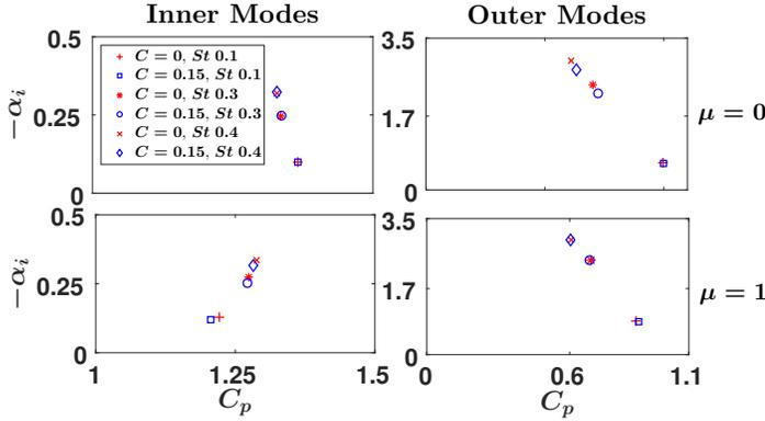
**Figure 2: Eigen spectrum for  $C = 0$  and  $C = 0.15$  cases plotted for three different  $St$  (0.1, 0.3 and 0.4). Left column represents inner modes and right column represents outer modes. Only first two dominant azimuthal mode ( $\mu = 0$  and 1) traverse is shown for variation in  $St$  and  $C$**
