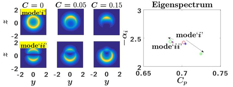
**Figure 3: Outer modes pressure eigen function plots for concentric ( $C = 0$ ), intermediate ( $C = 0.05$ ) and partially eccentric ( $C = 0.15$ ) jet at  $St = 0.3$ . First row represents mode 'i' and second row represents mode 'ii' showing  $\mu = 0$  and  $\mu = 1$  mode characteristics respectively. Eigen spectra shows their respective traverse with increasing  $C$**
