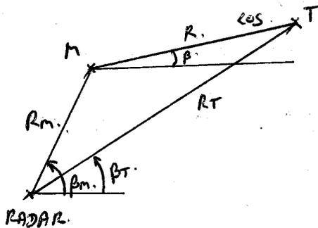
Pursuit guidance: Pursuit guidance requires the missile velocity vector to be always pointed towards the target. Hence, the <sup>missile</sup> velocity vector is along the LOS, that is,
