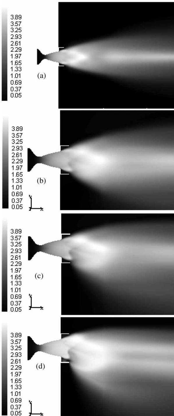
**Fig. 6** Mach no. distribution in the pitch plane with different vane deflections: (a)  $0^\circ$ ; (b)  $8^\circ$ ; (c)  $16^\circ$ ; and (d)  $26^\circ$
