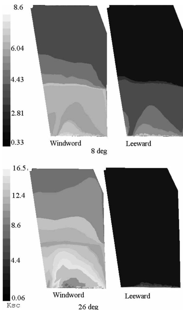
**Fig. 8** Surface pressure comparison between the windward and leeward sides of the vane with different vane deflection angles: (a) 8° and (b) 26°
