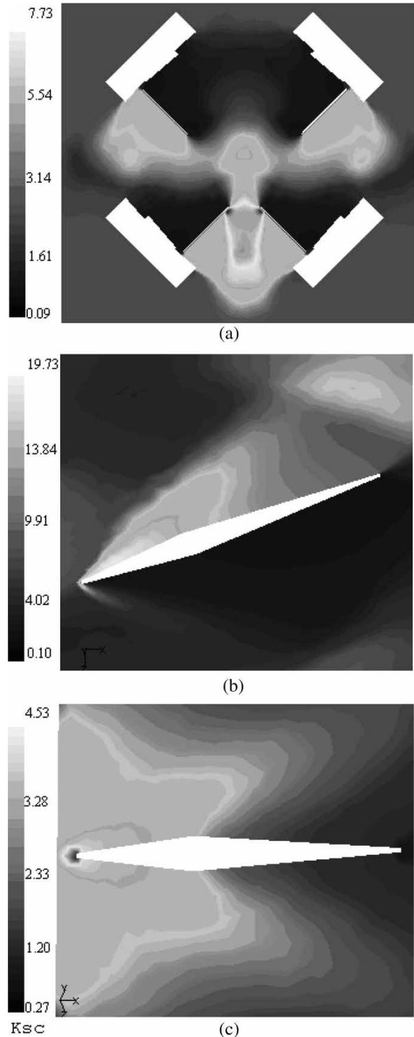
**Fig. 7** Blown-up view of the pressure distribution around the jet vane: (a) near the shroud; (b) around the deflected vane at  $26^\circ$ ; and (c) around the un-deflected vane
