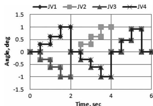
**Fig. 3** Normalized vane deflection history of four jet vanes
