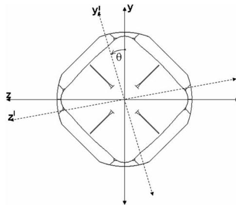
Fig. 12 Vehicle rear view showing rotational offset angle sign convention
