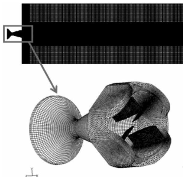
Fig. 5 Computational grid in the jet vane flow field
