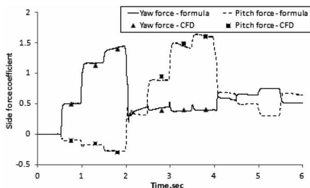
Fig. 13 Comparison of side force coefficient between the correlation and CFD data
