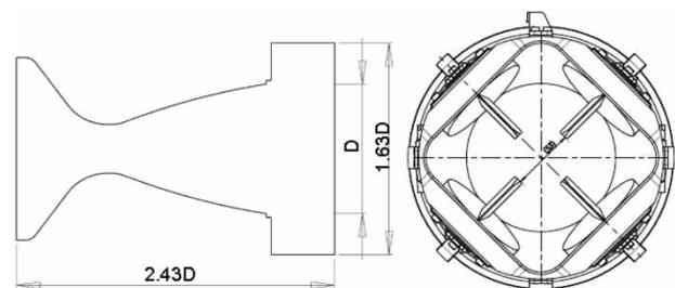
**Fig. 2** Arrangement of jet vanes at the exit of the nozzle
