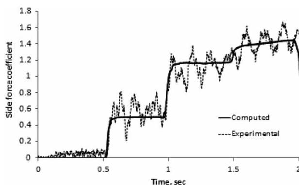
Fig. 14 Comparison of yaw force coefficient between theoretical correlation and experimental data
