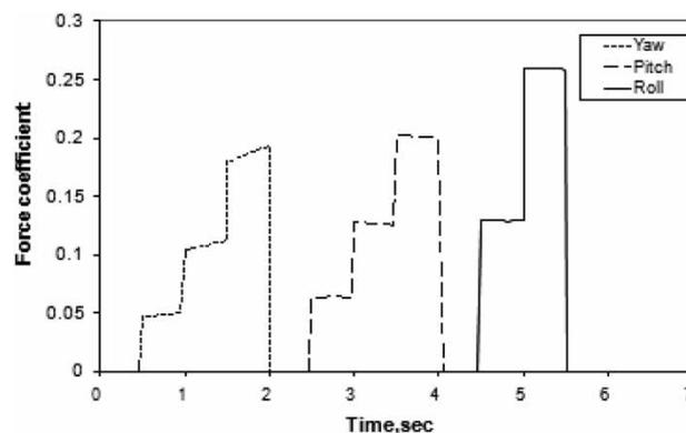
**Fig. 9** Variation of computed yaw, pitch, and roll forces with deflection angle
