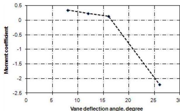
**Fig. 10** Variation of hinge moment coefficient with vane deflection angle
