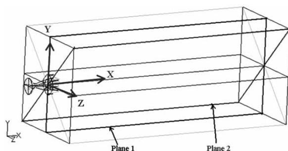
Fig. 4 Coordinate system and computational domain (Plane 1: passes in between jet vanes. Plane 2: passes through the jet vane)
