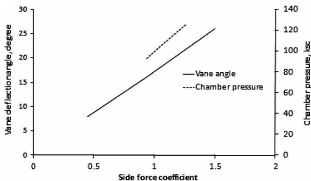
Fig. 11 Variation of side force coefficient with chamber pressure and vane angles
