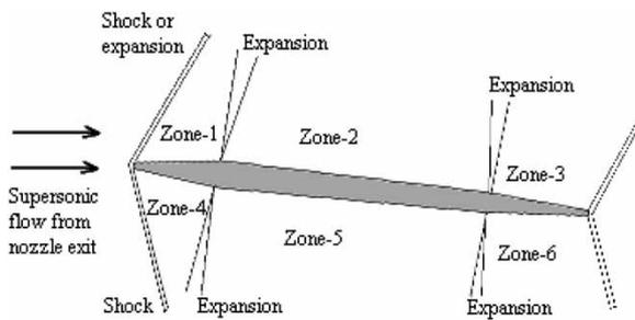
**Fig. 1** Typical shock structure for supersonic flow past jet vane-type geometry
