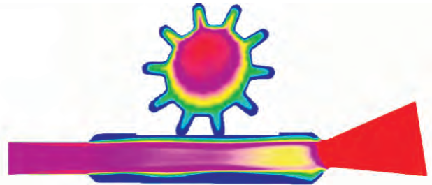
Figure 21. Mach number distributions in a solid rocket motor.
