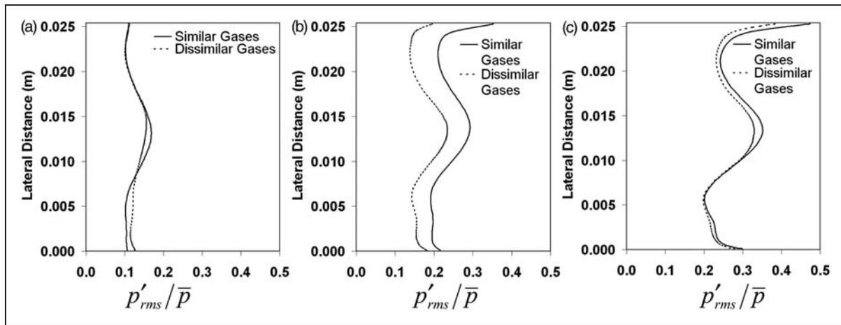
**Figure 5.** Pressure fluctuations for similar and dissimilar gases at an axial location of 400 mm: (a)  $Mc = 0.4$ , (b)  $Mc = 0.6$  and (c)  $Mc = 0.8$ .
