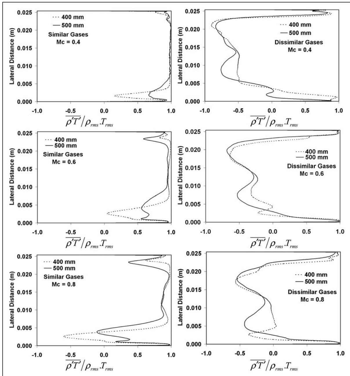
**Figure 7.** Variation of temperature density fluctuation correlation coefficient within the mixing layer at different  $M_c$  for both similar and dissimilar gases.
