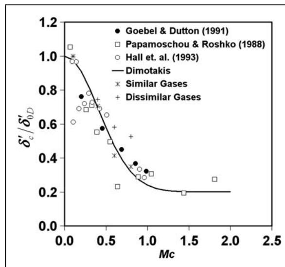
Figure 2. Normalised growth rate from different simulations compared with 'Dimotakis curve' and experimental data.
