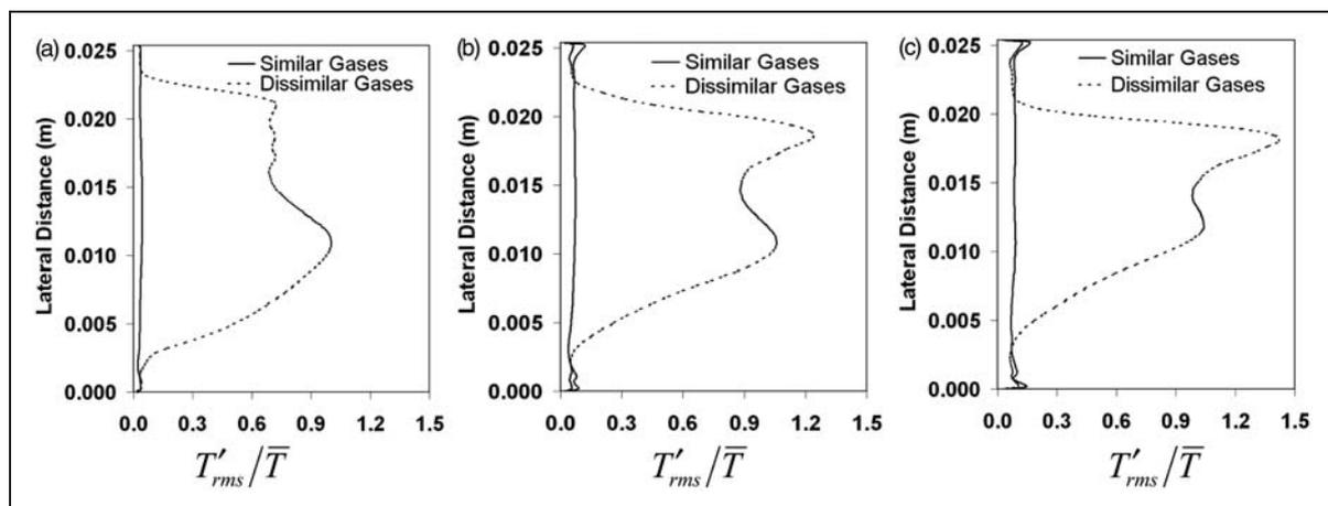
**Figure 3.** Temperature fluctuations for similar and dissimilar gases at an axial location of 400 mm: (a)  $M_c=0.4$ , (b)  $M_c=0.6$  and (c)  $M_c=0.8$ .
