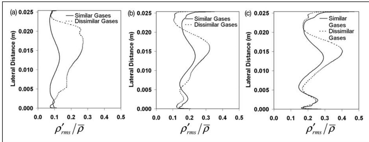
**Figure 4.** Density fluctuations for similar and dissimilar gases at an axial location of 400 mm: (a)  $Mc = 0.4$ , (b)  $Mc = 0.6$  and (c)  $Mc = 0.8$ .
