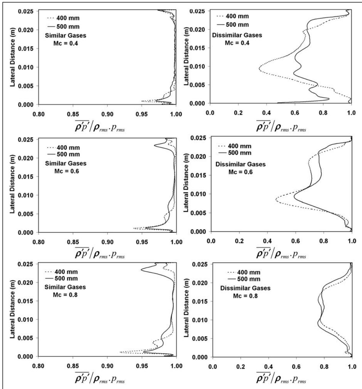
**Figure 6.** Variation of pressure density fluctuation correlation coefficient within the mixing layer at different convective Mach numbers for both similar and dissimilar gases mixing cases.
