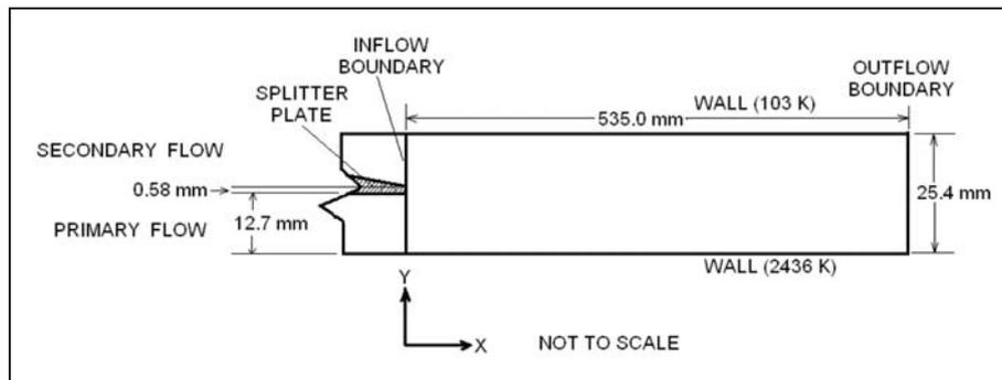
**Figure 1.** Schematic of experimental condition of Erdos et al.<sup>9</sup> for which simulation is carried out.
