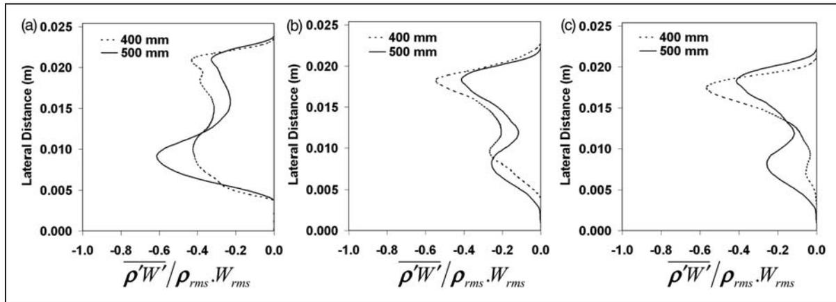
**Figure 8.** Variation of molecular weight density fluctuation correlation coefficient within the mixing layer at (a)  $Mc=0.4$ , (b)  $Mc=0.6$  and (c)  $Mc=0.8$ .
