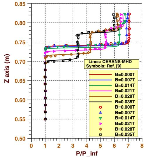
Fig. 5 Pressure profiles ( $p/p_{\infty}$ ) at  $x = 1$  m from intake ramp of various magnetic fields.
