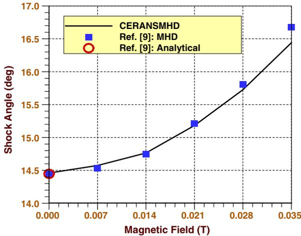
Fig. 7 Variation of shock angle vs magnetic field.
