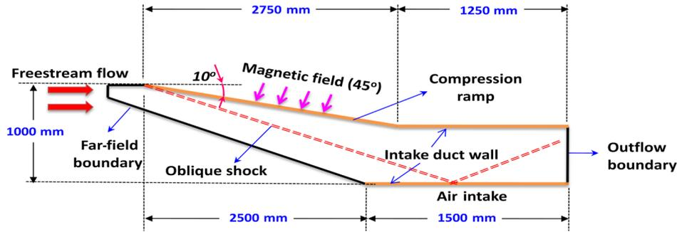
Fig. 3 Computational domain for MHD assisted air intake [9].
