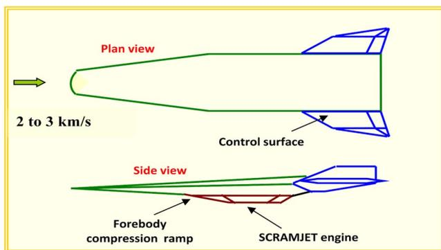
Fig. 1 Schematic of hypersonic scramjet cruise vehicle.
