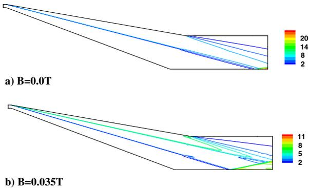
Fig. 4 Pressure contours, magnetic field variation study, Mach 10, and altitude of 40 km.
