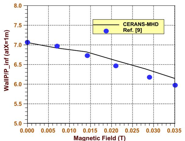
Fig. 6 Variation of wall pressure ( $p/p_{\infty}$ ) at 1 m location vs magnetic field.
