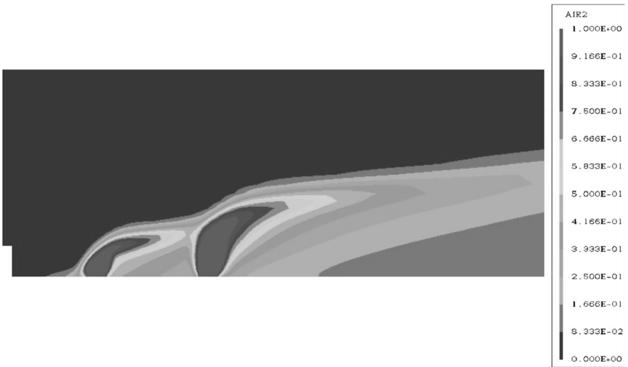
Fig. 5 Injectant mass fraction distribution ( y/D = 0.0 )
