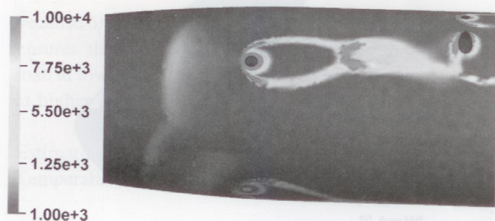
Fig. 9 Heat flux distribution on the missile body
