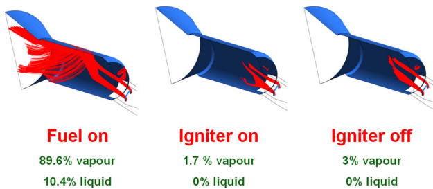
Fig. 4 Particle tracks for different conditions, percentage of kerosene vapour and liquid at the exit plane of combustor
