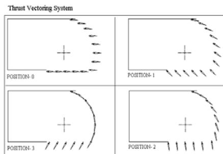
**Fig. 4 Louver profile vane thrust vectoring system**
