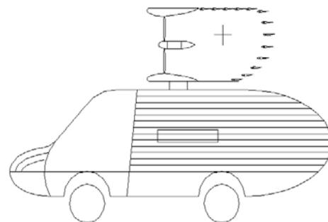
**Fig. 5: Set up for validating thrust vectoring system**
